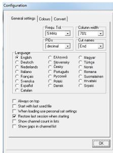
The value **Frequ. Tol.** (Frequency tolerance) is used when importing and indicates the tolerance a transponder frequency may have relative to the imported one to be considered to be the same. If you have for example a transponder with the frequency 11721 MHz in you settings and you import a channel with the frequency 11720 MHz and the frequency tolerance is set to 5 MHz no new transponder is created. This tolerance is also used for the transponder list.
